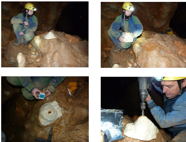
Supplementary Figure 7: Construction of a ceramic replica stalagmite to replace a removed sample. A drip logger was also placed inside the replica. Work performed by D. Sokolnikov (top) and A. Osinzev (bottom right). The stalagmite replica was later painted in brown to make it the same colour as the surroundings.
